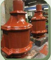
Upon arrival into our Derbyshire workshop, the hoppers were shot blasted and fully crack tested, before the cracked hopper was fusion welded using our Lloyd's approved procedures for cast iron. The two new spigot sections were manufactured and welded in place, before all repairs were ground to the
