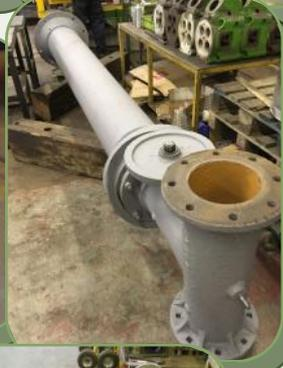
A main component which was missing was the elegant "swan neck" – the section which sits on top of the column and extends horizontally to carry water from the column to the loco tank. Again, a pattern was made and the swan neck cast, before machining and aging. We also redesigned and manufactured the finial and bracing which allows the counter-balance and swan neck to swing in any direction effortlessly.
