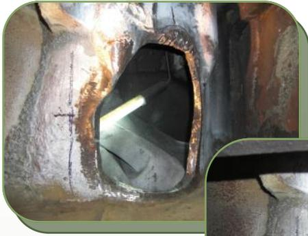
The hole was dressed to the correct profile to accept the new iron patch into the original block and then stitching work began.
