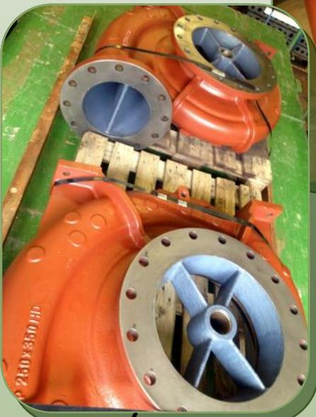
A world-wide Marine company requested our urgent specialized services whilst in dry dock to repair and recondition two fire pumps which had sustained severe cavitation in the main volute casings.
